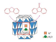
**Sift fluorene into a bowl**: Manganese oxide octahedral molecular sieves (OMS-2), with the overall composition KMn<sub>8</sub>O<sub>16</sub>·n H<sub>2</sub>O, catalyze the mild, green, and efficient oxidation of 9H-fluorene to 9-fluorenone. The involvement of lattice oxygen species has been implicated in a free-radical chain mechanism. In terms of reaction kinetics, the breaking of the C–H bond is rate controlling.
